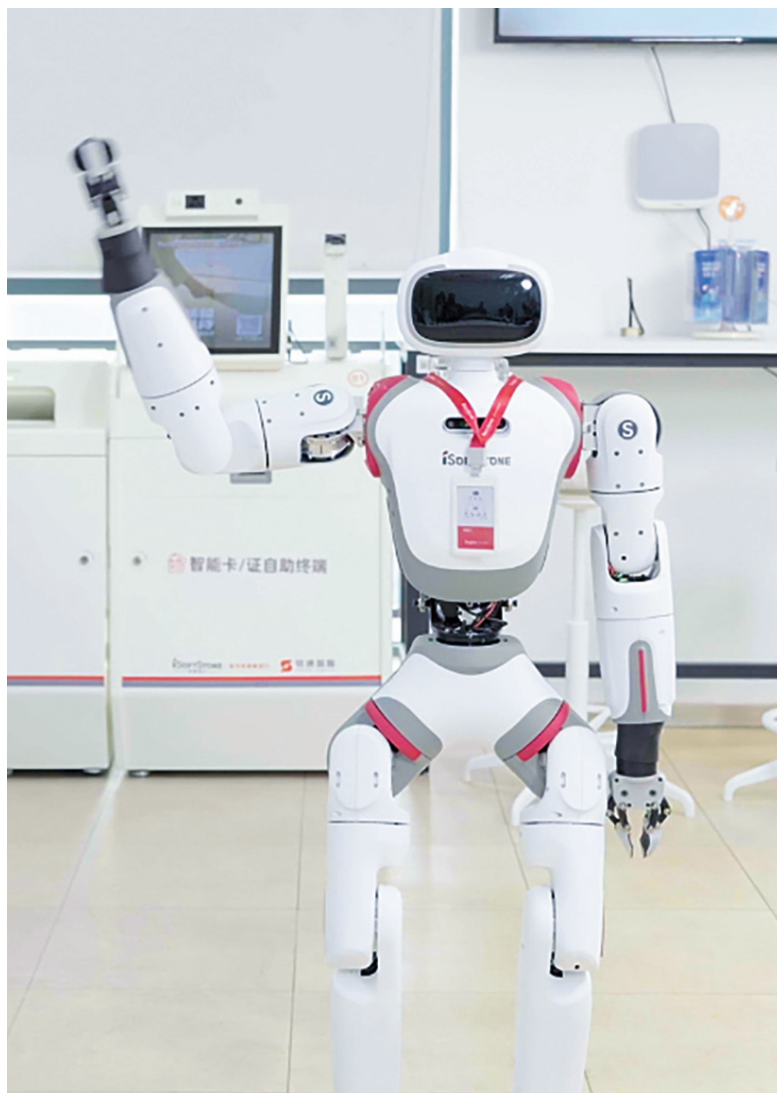
Tianhe C1 is a 130cm, 32kg humanoid robot, designed for research, education and interactive services. — Li Pin
